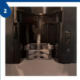
When putting the reservoir back, please ensure the clear component (above) is pushed down to the bottom of the tracking.
