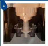
Ensure that the ridge on the pump is located on the uppermost ledge, as illustrated above.
